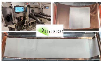
PLD process - Li on Cu: 5-10µm thin → a possible benefit to commercial foil (picture taken by Pulsedon)
